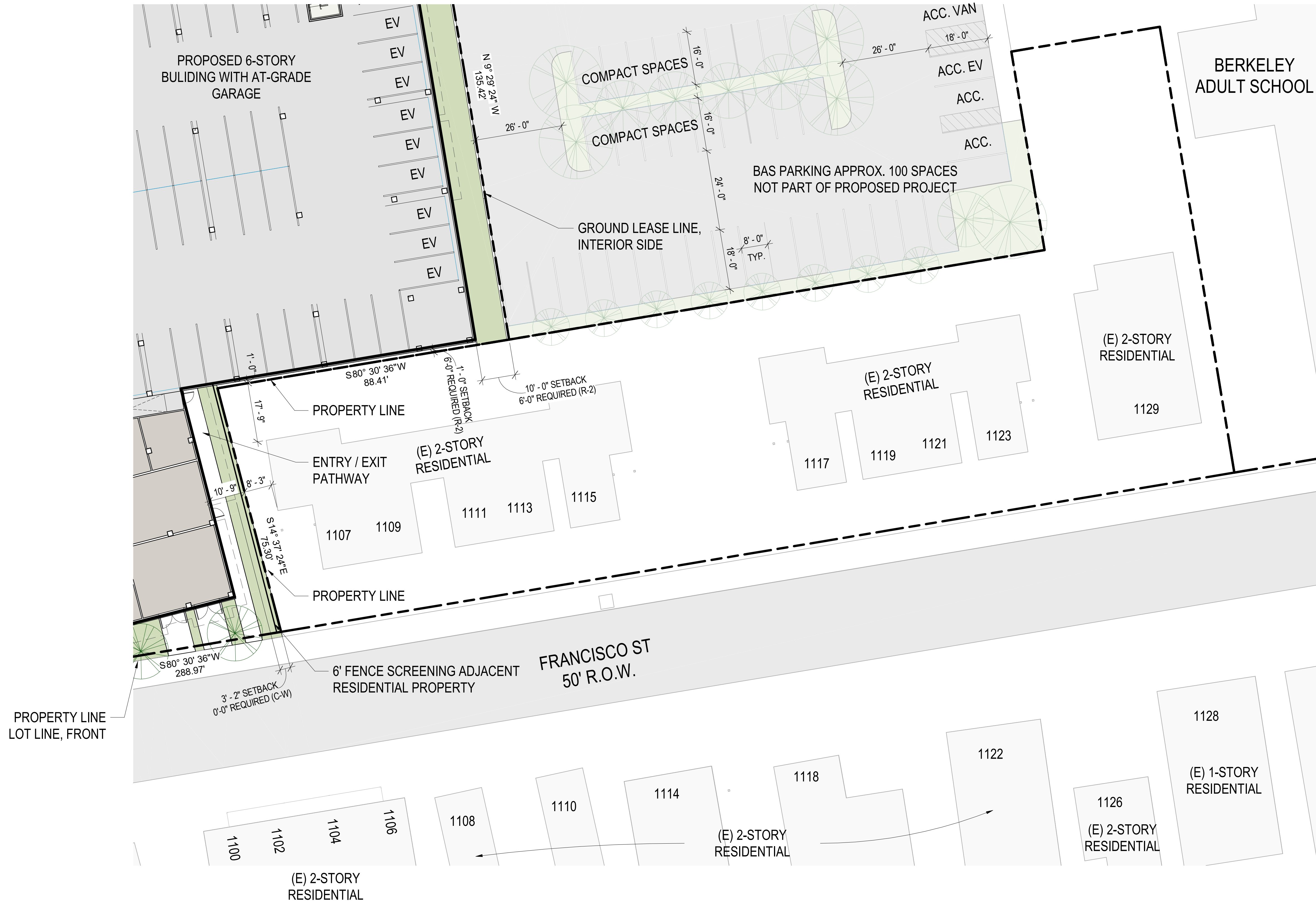
ENLARGED SITE PLAN - SOUTHEAST ① 1/16" = 1'-0"
