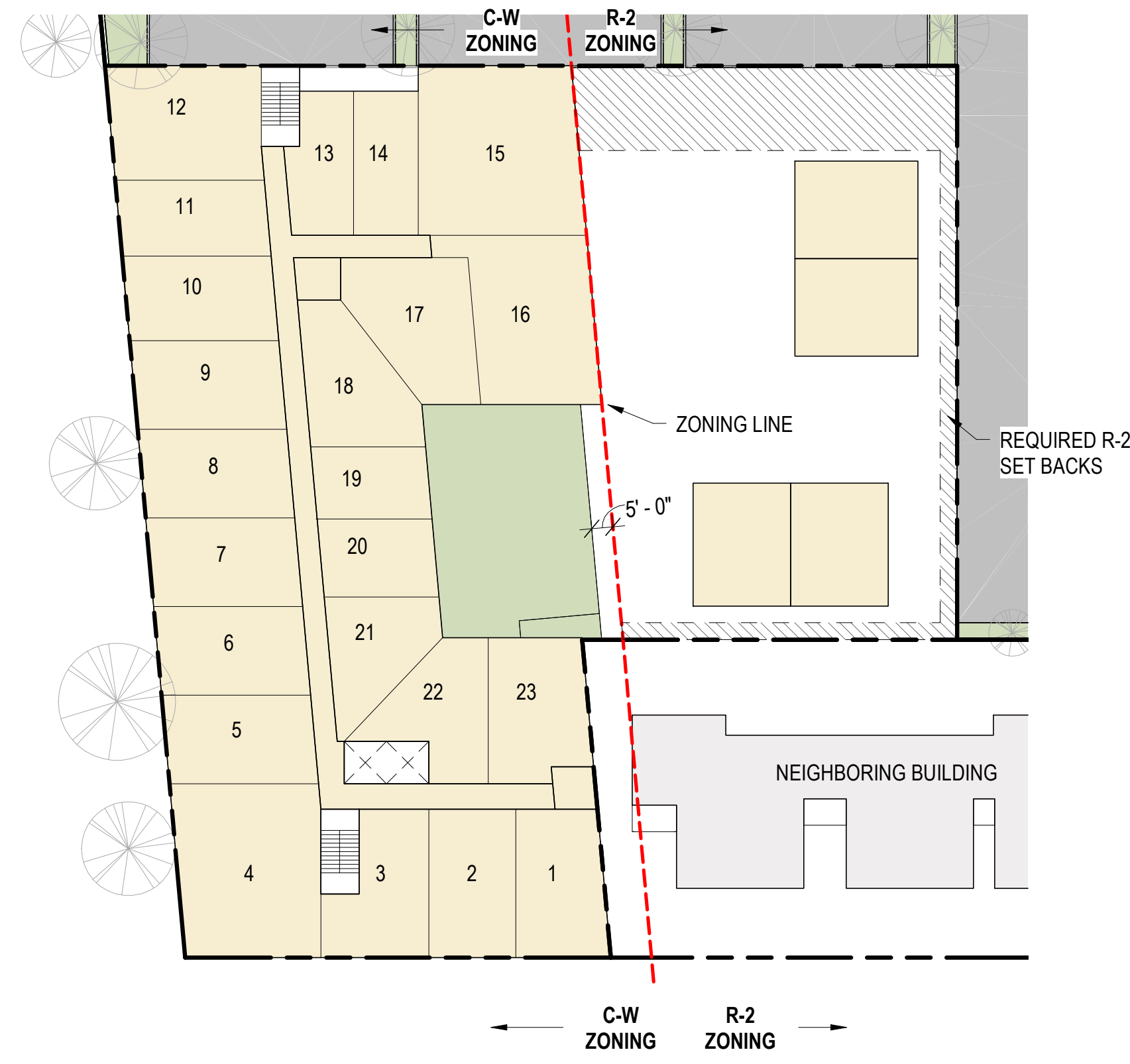
BASE SCHEME PLAN - LEVEL 2
