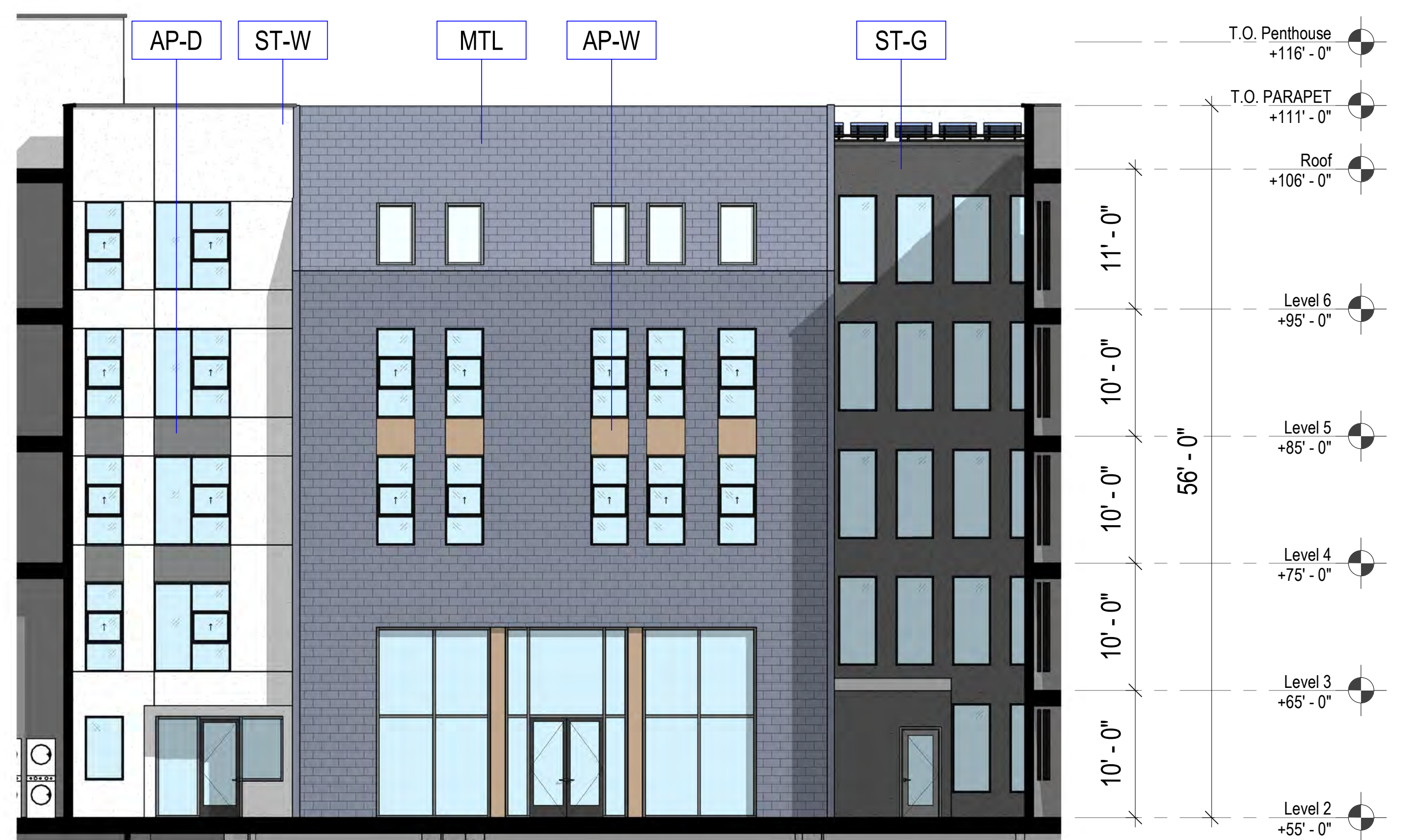
WEST COURTYARD ELEVATION 1 1/8" = 1'-0"
