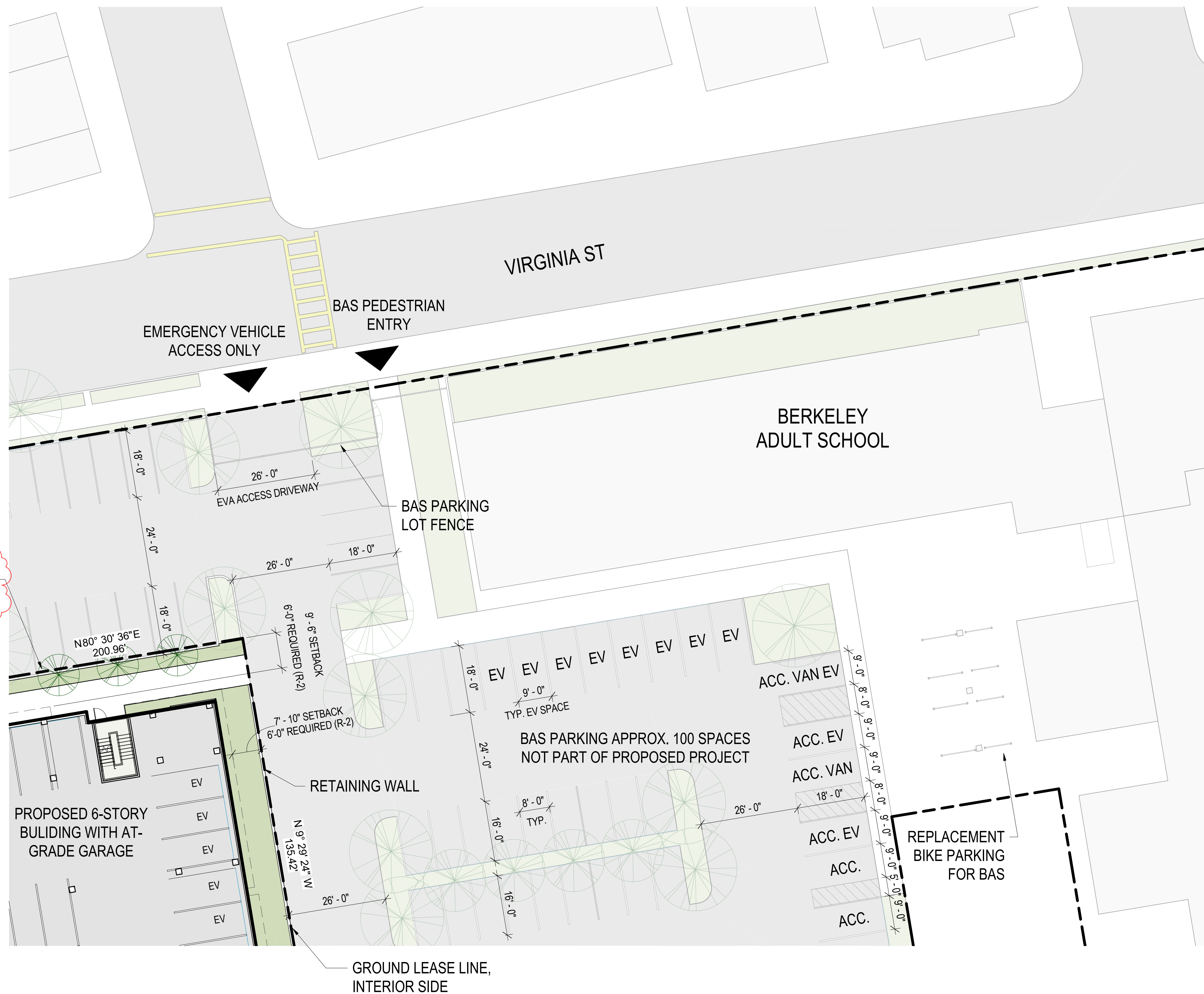
ENLARGED SITE PLAN - NORTHEAST 1/16" = 1'-0" ①
